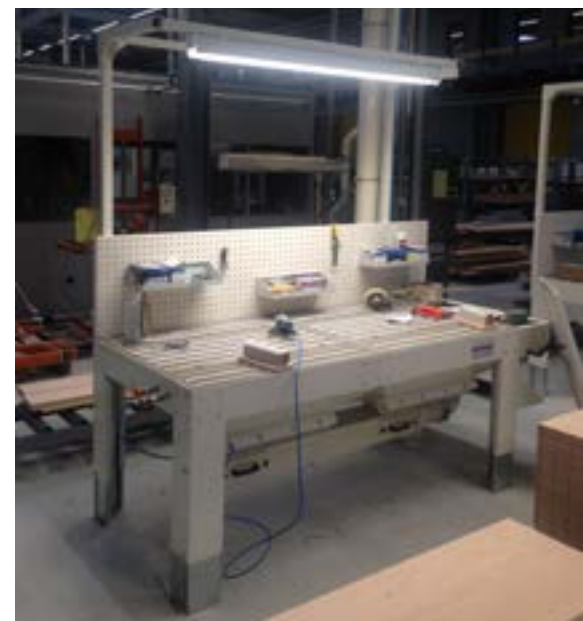
Expert Z20 dust extracting workbenches with lighting option in practical use
