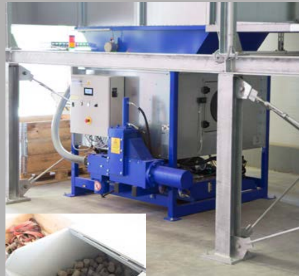
A MultiStar filter system with a BrikStar C briquetting press at a manufacturer of corrugated board packaging.
