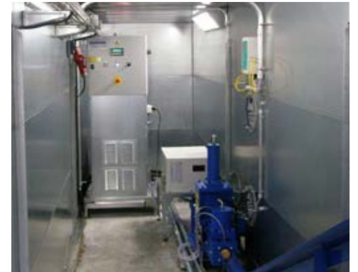
A BrikStar V model in a combination insert with a moving floor container and a MultiStar filter system. The arrangement in a weather protection cabin allows comfortable access. With water pliers cooling for continuous operation.
