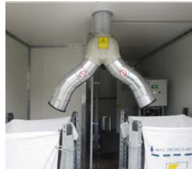
Briquette storage in Bigbag double container with frame and change over device. Switching possible according to preset briquette quantity.
