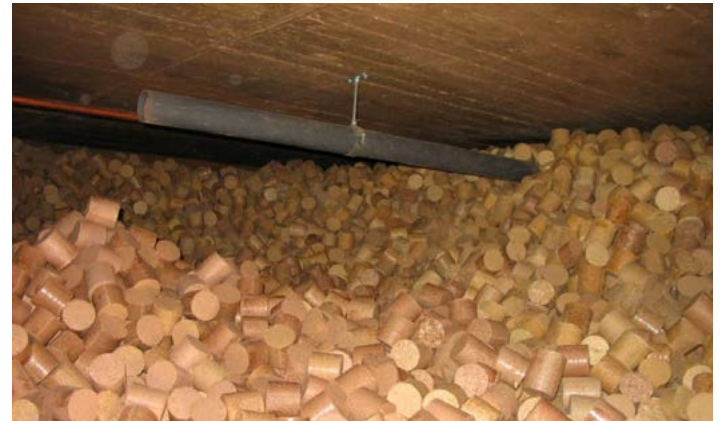
Wood briquettes are a high-quality, carbon-neutral fuel with an energy content of up to 5.5 kW/h per kg
