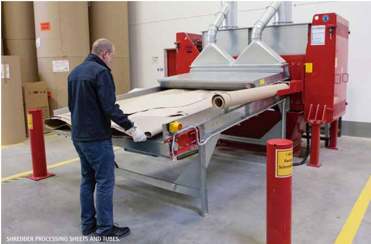
SHREDDER PROCESSING SHEETS AND TUBES.
