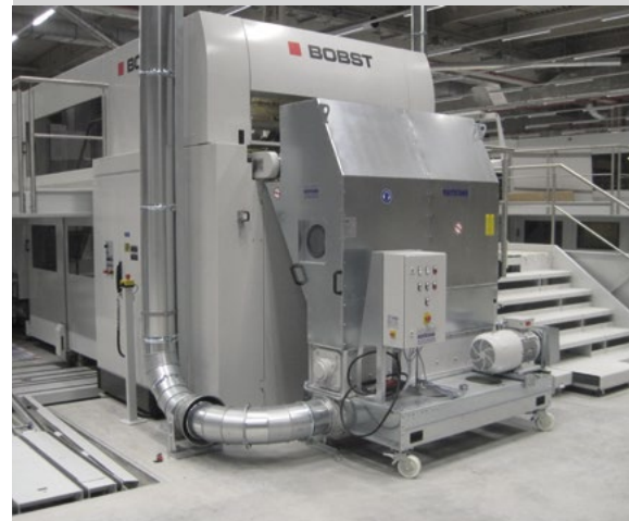
PHSS-K/G Shredder shredder for die cutting grid and gripper margin with docking station.
