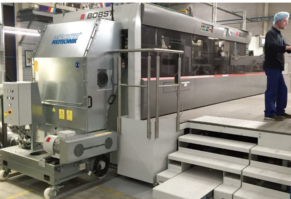
PHSS-K/G shredder Are specialized in their field of application and can be combined with any die cutter.
