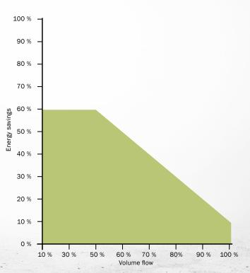
Conclusion: The greater the air volume and the greater the total pressure increase and the greater the control leeway, the greater the cost savings. The graph on the right shows the savings potential of up to 60 % compared to unregulated systems without energy-saving sliders.
