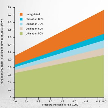
The graph shows the effect of frequency control in euros and cents. The higher the required pressure increase of the fans, the higher the energy costs per  $m^3$  of extracted air volume. But also the savings potential through the use of frequency converters when the system is only partially utilised increases with increasing pressure increase.
